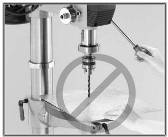
Figure 2. Never drill, holding workpiece by hand.
